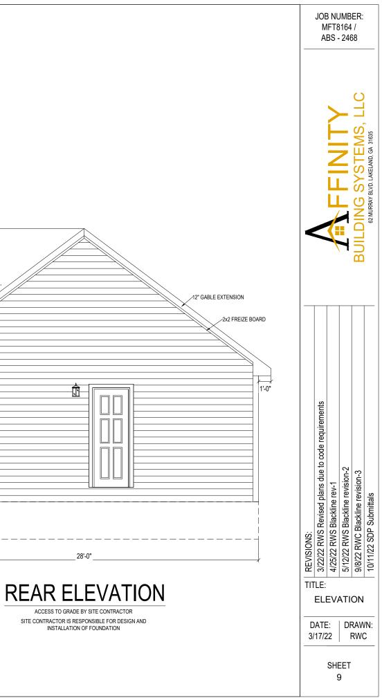
ACCESS TO GRADE BY SITE CONTRACTOR SITE CONTRACTOR IS RESPONSIBLE FOR DESIGN AND INSTALLATION OF FOUNDATION
